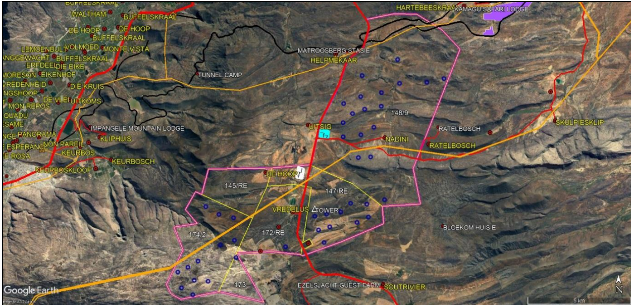
Figure 3.7: Hugo WEF site (pink) and constituent properties (yellow) in relation to proposed infrastructure: turbines (blue circles), and construction and operational terrains cluster Preferred (white fill) and Alternative (blue fill) sites. Also indicated are key roads (red), railway lines (black), Eskom lines (orange), and operational Touws River PV (purple fill)
